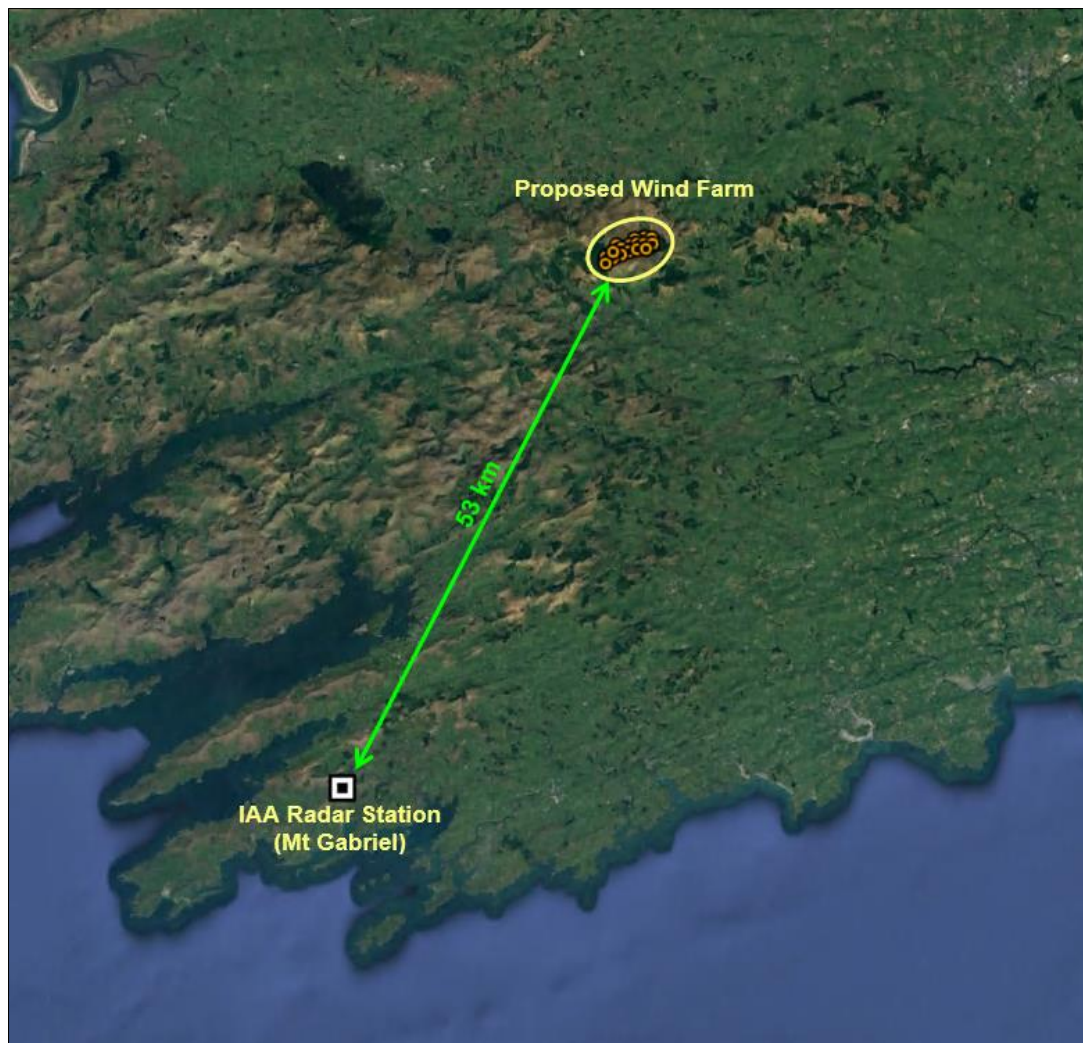
Figure 10. Radar Surveillance Site(s) relative to Cummeenabudodge Wind Farm.
